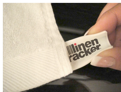
A Florida company's Linen Tracker device uses high-frequency identification tags to pinpoint the location of every towel, sheet and pillowcase in a hotel.
